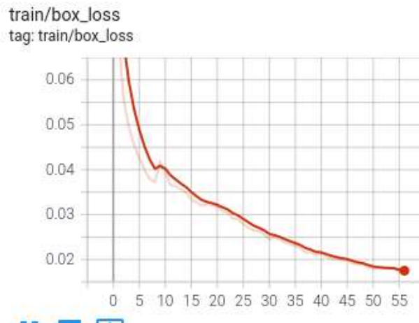
Figure 13. Training Box Loss Graph of Yolov8s.pt Model
